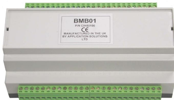
The BMB01 is an input and output control port (I/O) expander for ASL routers. The ASL VAR and VIPEDIA-12 Routers are able to support the connection of up to 9 remote BMB01 units, connected by a multi-drop RS485 serial interface.
